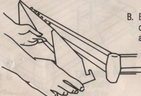
B. Bottom edge of gameboard rail fits onto protruding slotted supports at both ends of grandstand.
